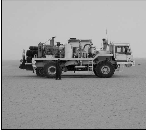
Figure 27.3: a) Vibroseis truck and b) geophones attached to cables at a desert base camp. Inset is a particle-velocity geophone that is about 9 cm long.
