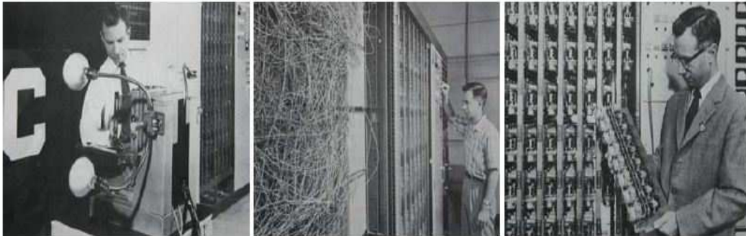
Figure 1.3: Mark 1 IBM computer for image recognition. Left photo: the camera system in which an input scene is recorded by a 20 \times 20 array of cadmium sulphide photocells to give an image with 400 pixels. Middle photo: the perceptron consisted of a patch board which allowed different configurations of input features to be tried. Right photo: racks of adaptive weights where the weight values were adjusted automatically by the learning algorithm. Images from Bishop (2006).
