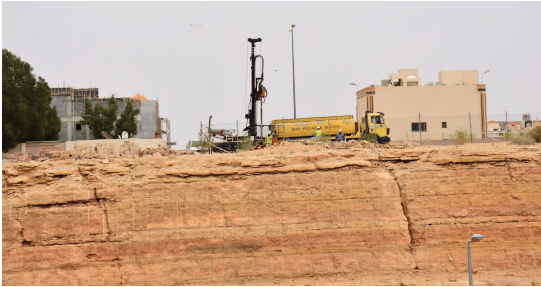
Figure 17.44: Drilling rig next to the carbonate outcrop (Ramdani, 2022). The core penetrates 35 m into the Upper Jubaila Formation in this outcrop.
