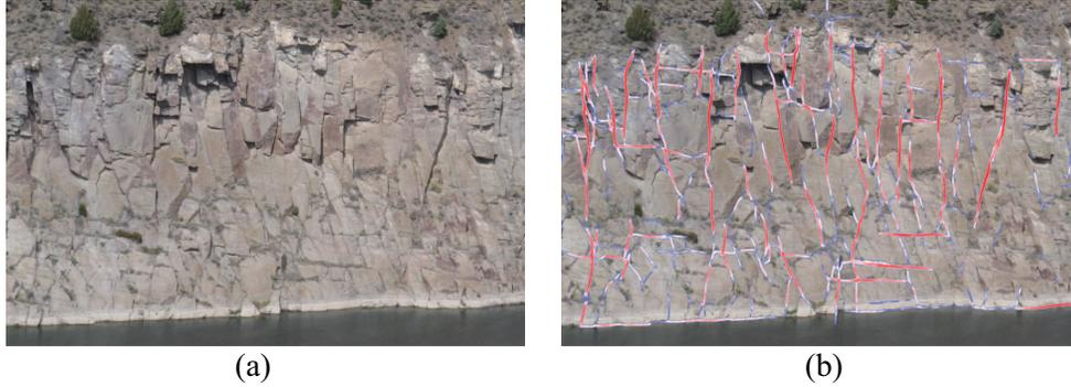
Figure 10: Crack detection of volcanic rocks at the Teton Dam Site, Idaho. a): near-vertical cooling cracks in volcanic rocks just downstream from the dam site; b): cracks labeled in red by U-Net. The red markings correspond to a probability between 0.7 and 1.0 in the softmax output, while the white-bluish markings correspond to a probability between 0.3 and slightly less than 0.7.
