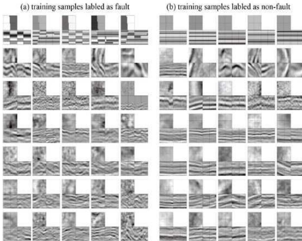
Figure 6.23: Samples labeled as (a) fault and (b) non-fault. All samples are randomly selected from the training dataset, except the first row showing synthetic samples. Each sample is composed of front, side and top panels which are inline, cross-line and time slices, respectively. The size of each slice is  $24 \times 24$ . The spatial grid size is 25 meters while the vertical time sampling interval is either 0.002 or 0.004 seconds for different cubes. Figure adapted from YXiong et al. (2018).
